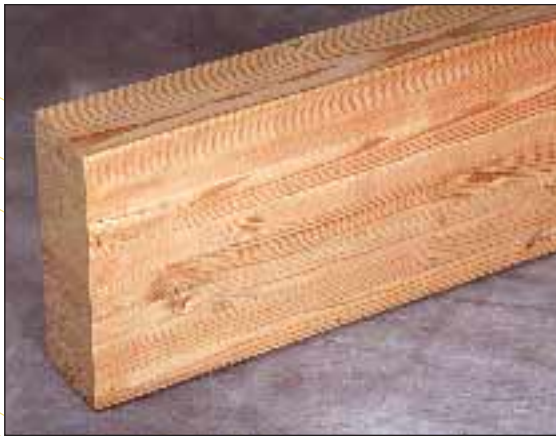
Close up of a glulam beam (Note the layers of laminated lumber.)
