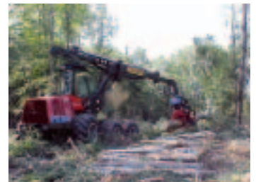
Harvester using its processor head to prepare logs.
