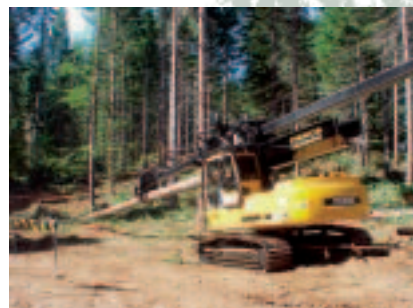
Mechanical delimiters delimb, top and buck tree into log lengths.
