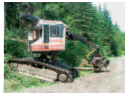
A tracked harvester demonstrates its agility in sloped conditions. Its multipurpose harvesting head can cut, top, delimb, buck, and stack a tree all in one motion.
