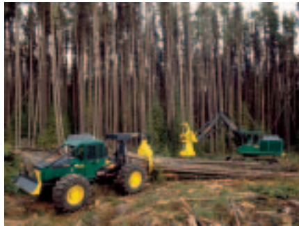
Wheeled grapple-skidder and feller-buncher working in tandem
