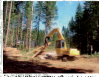
A hydraulic log loader equipped with a cab riser, special log boom, and grapple.
