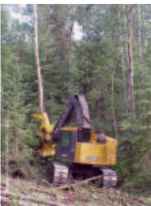
A feller-buncher is able to do harvesting work quickly and more productively while keeping the operator protected.
