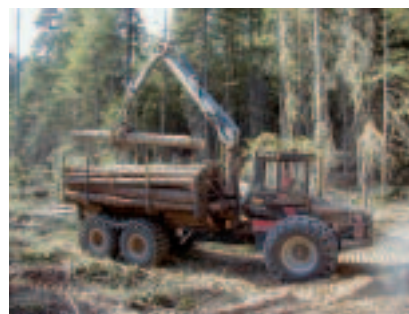
Forwarder loading cut logs for transport
